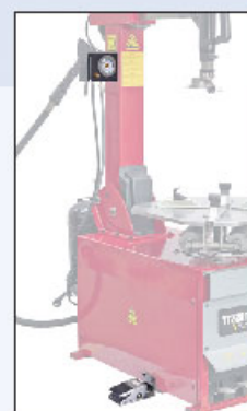
Pedal-controlled inflator 脚踏控制打气表
