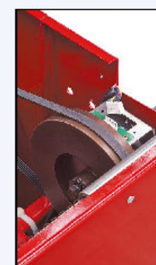
Pluggable position pick up board 插拔式光电板
